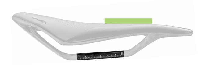
5. Tighten rail clamps to the recommended torque specification of the seatpost.
